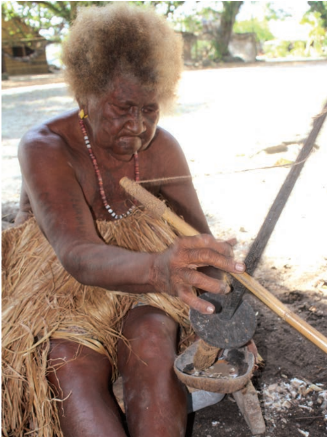
3 Drilling This is the oga process, drilling a hole at the centre of each shell bead using a home-made drill.
